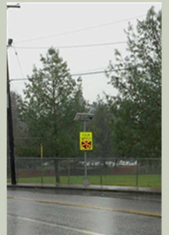
Driver feedback signs provide real-time information of a driver's speed and reminds drivers of the posted speed limit.
